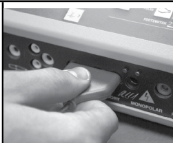
Figure 2. Plug the 3-prong power cord into the electrosurgical generator of your choice, (Figure 2). Confirm that all power settings on the generator are appropriate for the procedure being performed. The electrosurgical generator's intensity should be set as low as is necessary to achieve the desired effect. PlumePen® Ultra is a monopolar electrode, the use of a dispersive electrode is required to prevent burns/injury to patient. Please refer to electrosurgical generator user manual and dispersive electrode instructions for use for additional instructions.
