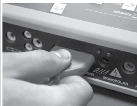
Figure 2. Plug the 3-prong power cord into the electrosurgical generator of your choice, (Figure 2). Confirm that all power settings on the generator are appropriate for the procedure being performed.
