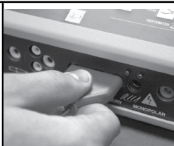
Figure 2. Plug the 3-prong power cord into the electrosurgical generator of your choice, (Figure 2). Confirm that all power settings on the generator are appropriate for the procedure being performed.
